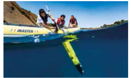
Deploying and recovering the glider from small boat
